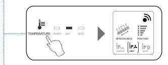
Press "TEMPERATURE" button twice, "DRY " light is on, and (included light) icon on the screen lights on, then adjust wind temperature by "+", "-" button. It is regarded as operation completed if there is no operation in 5 seconds, and then "DRY" light is off, ( ) icon disappears. Long press "-" button until the "DRY" icon disappears to close the "DRY" function.
