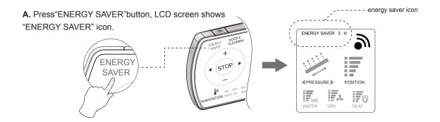
**B.** Press"ENERGY SAVER"button again, LCD screen shows figure "6", and the "ENERGY SAVER"icon disappear after 3 seconds, the setting succeeds. The toilet enters the energy saver mode from 9:00 to 15:00 every day. During this period, power light is off, and the energy saver light is on. It goes back to normal operation mode after energy saver time.
