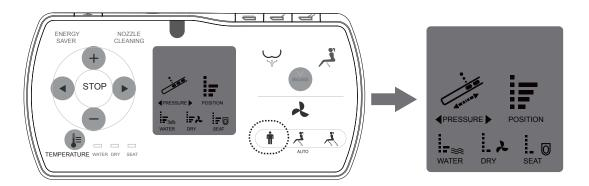
For example, the nozzle position is on level 2, and massage function is open; the water pressure is on level 4; water temperature is on level 2, while dry temperature and seat temperature are on level 1.
