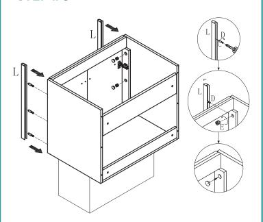
Install screw part D on the fron legs, Put the legs on the cabinet and screw the cam-lock E tightly, re-cover the decorative hole cover on the panel.
