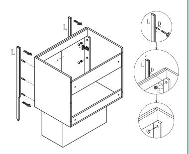
Install screw part D on the fron legs, Put the legs on the cabinet and screw the cam-lock E tightly, re-cover the decorative hole cover on the panel.
