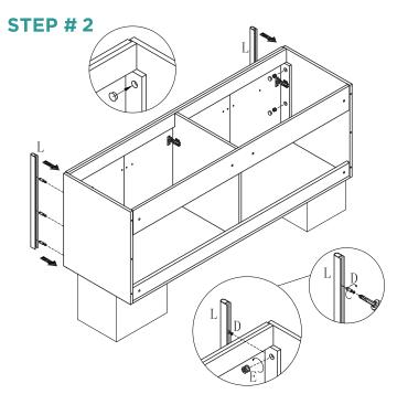
Install screw part D on the fron legs, Put the legs on the cabinet and screw the cam-lock E tightly, re-cover the decorative hole cover on the panel.
